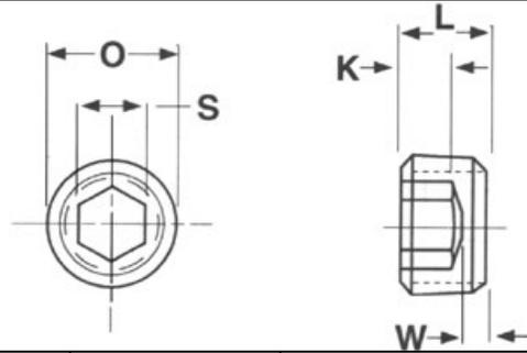
Note: "3/4 Taper" and "7/8 Taper" fit into the same hole. The "3/4 Taper" will stick up out of the hole a bit, the "7/8 Taper" will be Flush.
